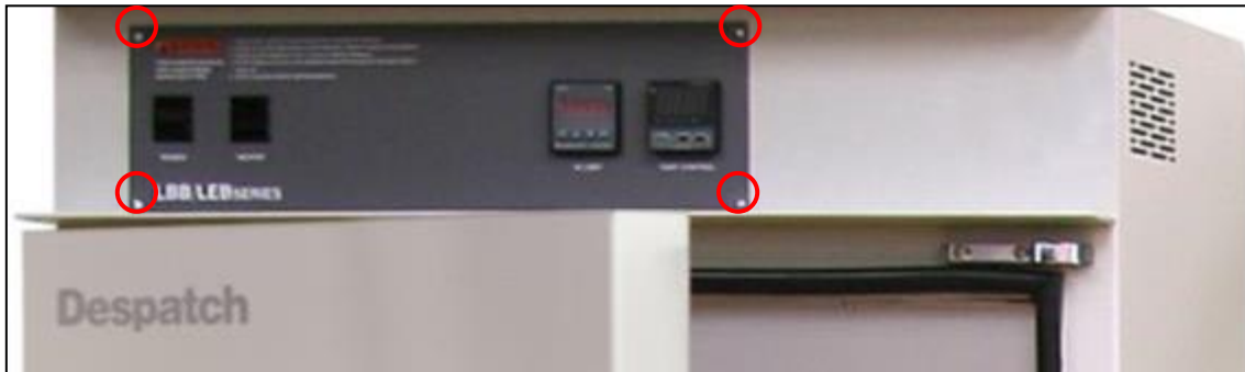
Figure 13. Remove Control Panel to Access Control Instrument (using T20 Torx bit driver).
