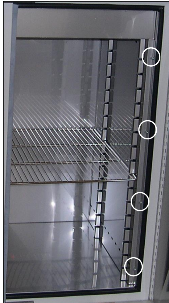
Figure 21. Remove Screws to Remove Each Duct (using T15 Torx bit driver).
